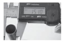
The calliper shows that the diameter is 15.10 mm.
